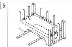
5. Using two pieces of lumber placed under the tub to protect the floor, slide tub into place, remove the 2 pieces of wood and lower tub into place, using metal shims level tub. It may be necessary to move tub in and out if no access is available from the back or sides in order to install shims.
