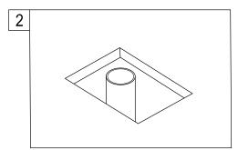
Determine the tub drain location, cut an opening; opening should be a minimum of 6" x 15".
