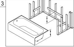
3. Measure the distance from the floor to the underside of the tub deck, using this measurement install 2" x 6" lumber stringers on all 3 sides, top surface of the stringer should be at the height of the underside of the tub deck.
