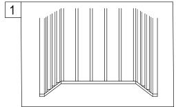
1. Prepare area by framing the area where the tub will be installed, make sure to check that everything is square, plumb and level.
