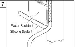
7. Install water resistant gypsum board and finish surface material (tile, stone) and seal all edges with silicone caulking to prevent water damage.
