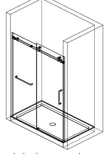
15. Clean all the surfaces where the shower door or the hardware meets the surface of the shower base or bathtub and apply a generous bead of clear silicon caulking, wipe off any excess.
