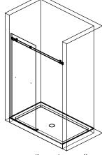
8. Insert stop blocks (E) onto the top rail and insert the top rail on the wall brackets (A) secure top rack to the Fixed glass panel by threading and tightening the fixed panel fasteners (B).
