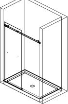
9. Insert the bottom guide (J) onto the lower rail (I) and secure it with self-tapping screw, do not tighten.
