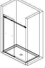
7. Remove top rail (D) from fixed glass panel and secure wall brackets (A) at the marked location by using anchors and screws.
