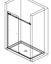
10. Lift sliding panel and place rollers on the top rail (D) while at the same time inserting the panel on the bottom guide. Insert the door panel guards (P) on the two holes below the rollers and thread, make sure to install the longer most protruding portion to the outside, do not over-tighten.
