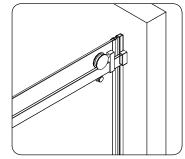
12. Attach the water sealing gasket (M) to the fixed panel.
