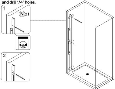
3. Insert anchors (aa) and gently tap using a rubber mallet, add a bead of silicone to the back of the U rail place the fixed panel rail at the desired location and secure with the enclosed screws (bb)
