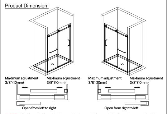
**NOTE:** The installation of right or left door of this model is interchangeable. The installation diagram of the left swing door is shown in this manual. For the installation of the right door, start from the opposite wall and reverse the direction of the installation steps.
