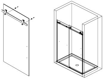
11. Using screws and after applying a bead of silicone to the back, attach the U channel at the location where the sliding door meets the wall. Insert magnetic rubber seal into U Channel.
