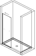
6. Attach wall brackets (A) to both ends of the top rail (D) and secure rail to fixed glass with the fixed panel fasteners (B), level top rail and mark the perimeter of both wall brackets (A).
