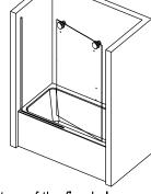
5. Slide lower rail (L) onto the bottom of the fixed glass panel and slide fixed glass panel onto the U channel (N), confirm that the fixed panel is level, you may need to add small shims, apply silicone caulking to secure lower rail.
