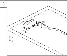
Insert plastic washer and flush arm through bracket, then place rubber washer onto bracket.
