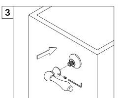
3. Position handle to the right or left depending on preference and secure by tightening set screw on the side of the handle or in certain applications it may have a screw in the center of the handle, after securing handle, placed decorative handle cap (certain models only) onto handle.
