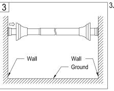
Holding the larger sized rod, rotate the smaller rod until it is locked into position securely.
