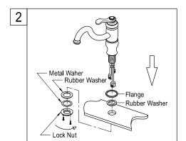
2. Set the faucet in place, insert the inlet shank through the sink hole, and press down. Assemble the washers and locknut on the inlet shank, and then tighten the nut with hand. Secure this faucet tightly onto the counter with the metal nut underneath the counter as shown on this diagram.
