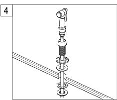
4. Attached sprayer head, to hose, and hand tighten only. Plumbers tape is not required. Drop sprayer hose through hose guide and let it rest in place.
