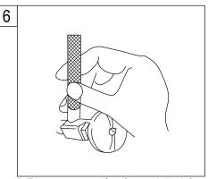
6. Turn on water supply valves and check for leaks, especially at hook-ups to supply lines.
