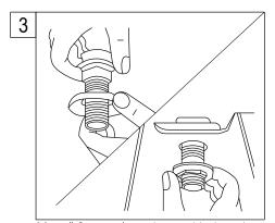
Install Sprayer: Insert hose guide through guide flange and snap into place. Install guide through sink and attach with mounting nut.
