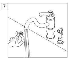
7. Remove the aerator before turning on your new faucet for the first time. This is to prevent any deposits from clogging your aerator. Allow both hot and cold water to run for one minute. Replace aerator.
