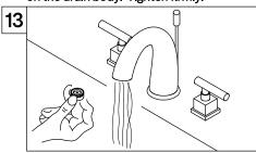
13. Remove the aerator, turn on the faucet, let water run for at least one minute, this will clear any debris left in the line, reinstall aerator.
