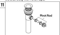
11. Place pivot rod into pivot rod opening. Slide pivot nut over pivot rod and thread it on the drain body. Tighten firmly.
