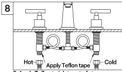
8. Apply Teflon to inlet port of stem assembly and thread supply lines (not included).
