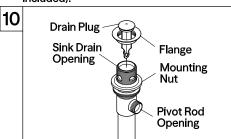
10. Apply silicone to bottom side of flange. Install flange body up through the drain opening, hold the drain flange body in position with pivot rod opening facing the back of sink and hand tighten the mounting nut. Be sure to clean excess silicone.
