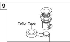
9. Thread mounting nut and bottom gasket onto drain body. Wrap top threaded end of the drain body with Teflon tape.
