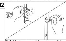
12. Guide the pivot rod through one of the holes on the lift rod strap and secure it with the spring clip. Then adjust the height of the lift rod by resetting the clevis screw. With lift rod in position on the faucet, insert lift rod through lift rod strap and secure with the clevis screw.
