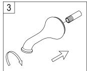
3. Slide the spout over the pipe. With the spout tight to the wall, tighten the set screw to the pipe.
