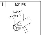
1. The stub-out pipe for spout installation must be at the length illustrated measured from the finished wall surface.
