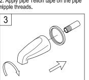
3. Slide the spout and flange over the pipe. With the spout tight to the wall, tighten the set screw to the pipe.
