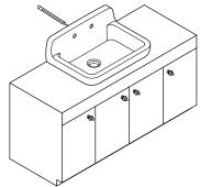
Set the sink at the desired place and mark a horizontal leveled line at where the top of the backsplash will be situated, remove the sink, place template on the wall and align the leveled line, making sure that the sink front is parallel to the front of the counter. Be sure the sink is properly centered, both front to back and side to side.
