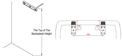
Mark the position of the holes, if the sink will be secured to wood bracing behind the wall, secure bracket using 3" wood screws, drive in and tighten up the wood screws at the marked locations to secure the bracket onto the wall.
