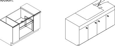
Place template on the countertop, making sure that the sink front is parallel to the front of the counter. Be sure the sink is properly centered, both front to back and side to side. Check for adequate clearance relative to cabinet walls and pull-out or tilt-down drawers. Tape the template in place. Trace around the template.
