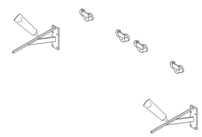
6. Install faucet, supply lines and drain on the sink, place the sink on the wall at the location where it will be installed and slide down onto the wall brackets
