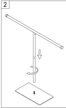
2. Place the base assembly on a level spot on the ground. Thread the free end onto the base assembly tightly in a clockwise direction.
