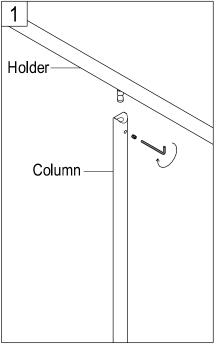
1. Install towel bar into the column, attach it securely by tightening the set screw with an allen wrench.
