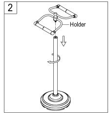
2. Install paper holder assembly onto the free end of the column tightly in a clockwise direction.
