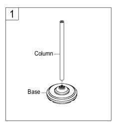
1. Place the base on a level area on the ground. Thread one end of the column onto the base tightly in a clockwise direction.
