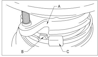
Lift and turn the Lower Mount Ring counter clock-wise until all three mount tabs lock over the Ridges
