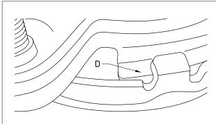
As the Lower Mount Ring is turned counter clockwise each tab slides up onto the Upper Mount Ring Ramp (E) and locks in position over the Ridges (F). Use a screwdriver or hammer for leverage if needed. If a disposal needs to be removed, tapping on the Ear clockwise
