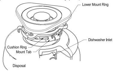
NOTE: Cushion Ring included between the Upper Mount Ring and Lower Mounting Ring.
